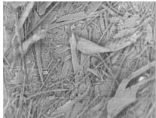
Plate II: SEM graph of treated feathers at 350x (760 μm)
